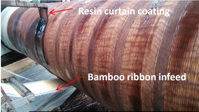
Pipe winding using ribbon and resin
